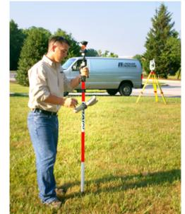
Leica Robotic TCRP 1203 Reflectorless Total Station
